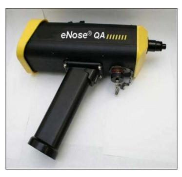
sensor array and associated software capable of making a determination of clean versus contaminated samples or leaks in ~3 seconds after pulling the trigger. The system provides ready, alarm, and self-test status via visual indicators (LED, LCD) and audible alarms.
